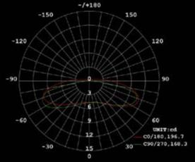
This is the only way you can have an RGBW LED module with more than 120-degree beam angle. The combination of the dotted dome and the bezel-free lens makes the light disperse evenly.
